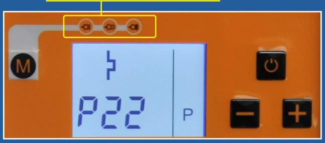
The flat parts program is ideal for the coating of panels and flat parts.
